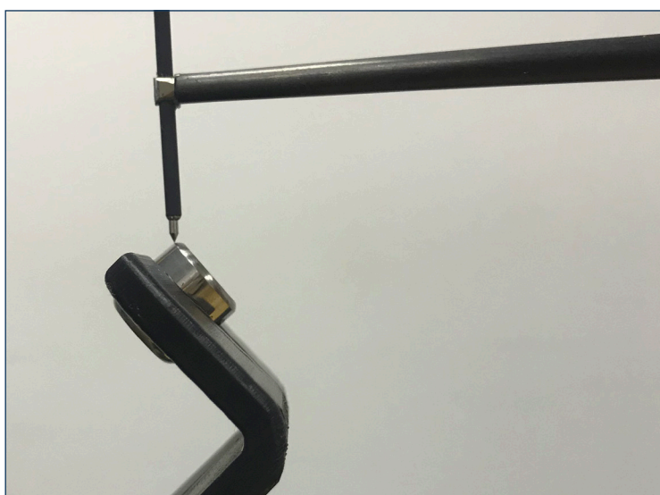
Figure 3 - Roller bearing angled at 45° allowing all 4 sides of the component to be measured in one setup and without external reference fixtures.
