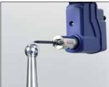
A simple automated routine that allows the user to set all axis positions without manual entry, removing operator error and ensuring positional consistency when programming.
