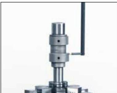
Follow mode is possible using the Radial Straightness Unit, this ability to track the surface of the part allows measurement of tapers, splines, camshafts, CV joints and much more.
