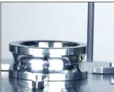
The world-leading gauge delivers 4 mm of range, twice the range of most roundness instruments. This enables the unique capability of roundness, contour, and roughness measurement from a single gauge.
